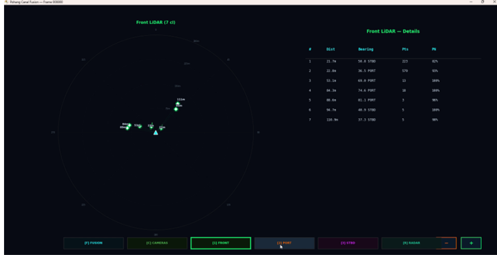
Fig: 4.2 The front LiDAR view for frame 008000 shows seven clusters that remained after applying PointNet filtering, with distances ranging from 21.7 to 110.9 metres.
