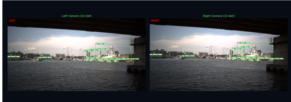
Fig: 3.2 YOLOv8 camera detection output on a Pohang Canal left-camera frame.
