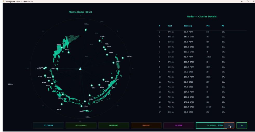
Fig: 4.3 Radar view demonstrating 28 confirmed radar obstacles at ranges from 479 to 1493 metres.
