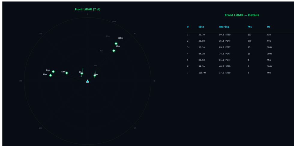
Fig: 3.6 LiDAR top-down view with PointNet-filtered clusters highlighted.
