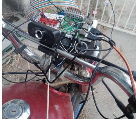
Fig 5.4: Camera Module Mounted on Handlebar — Rider View
