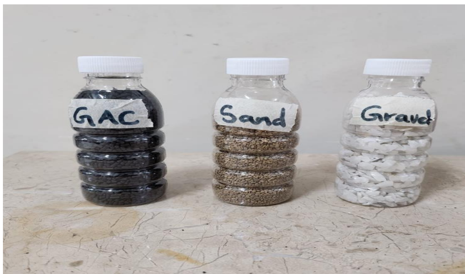
Figure 2.1: Prepared raw adsorbent media components (Coal-based Granular Activated Carbon, Pool-filter grade Silica Sand, and Graded Fluorite Gravel) stored in labeled containers prior to column packing.
