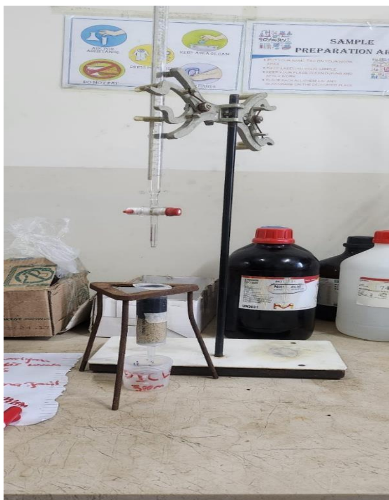
Figure 2.3: Complete gravity-driven experimental setup featuring an overhead glass burette for controlled influent delivery into the multi-layer fixed-bed adsorption column.
