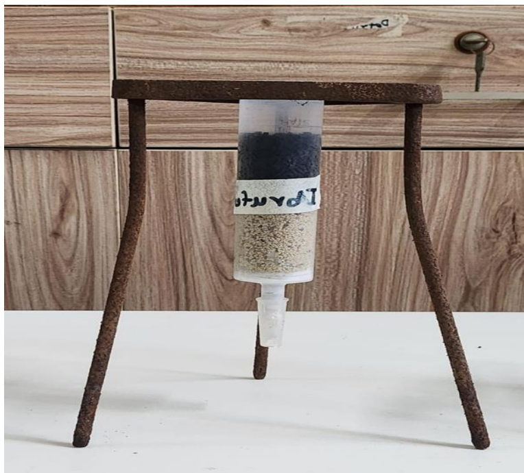
Figure 2.2: Assembled 60 mL multi-layer fixed-bed syringe column containing sequentially packed layers of cotton, gravel, silica sand, and GAC active adsorption zone.
