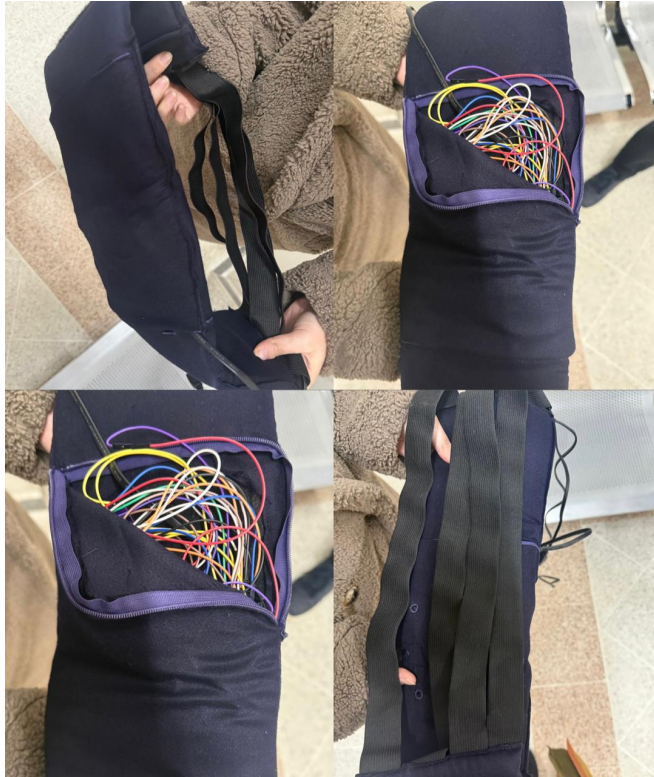
Figure 5.3: Hardware Behind the Fetal Monitoring Belt
